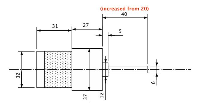
Kysan Electronics 1156007 Motor as base design New longer shaft without "D" shaped flat 1156007 Modifications Gear Motor File: gearmotor\_0.mdd Rev 0, M.L.Shaw, 21Jan2009 WindUpKey L.L.C.
